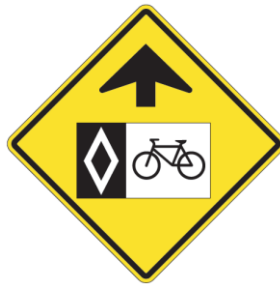
Reserved bicycle lane ahead 前面有为自行车预留的车道
