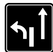
Left lane turn left, right lane straight 左线左转，右线直行
